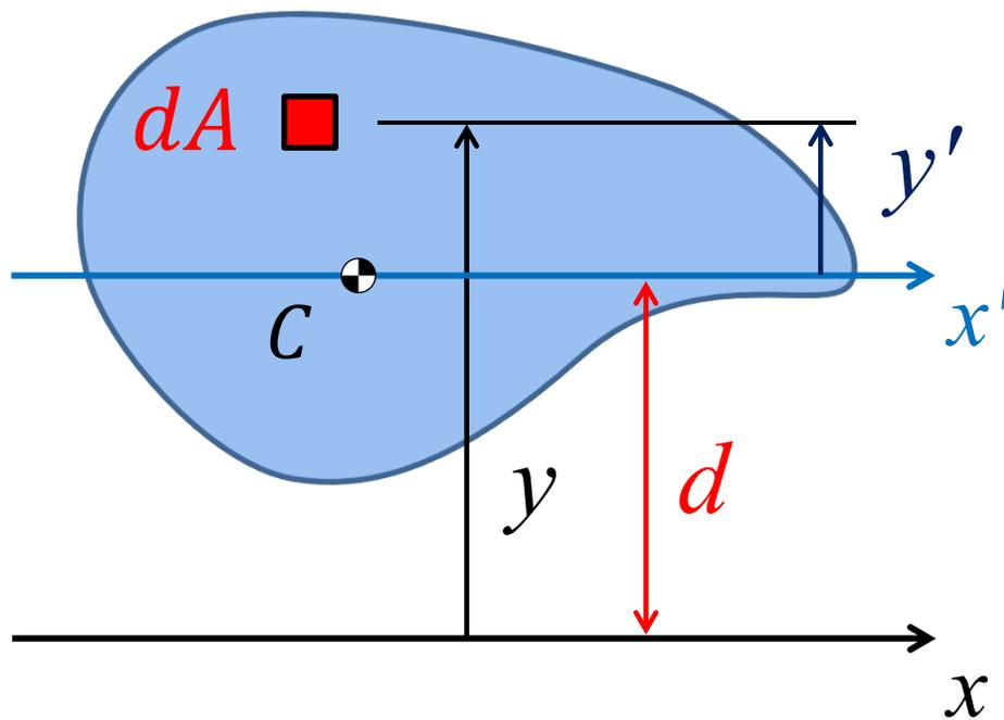
Consider an axis  $x'$  that is parallel to the  $x$  axis and passes through the centroid of the area. The distance between the two parallel axes is  $d$
