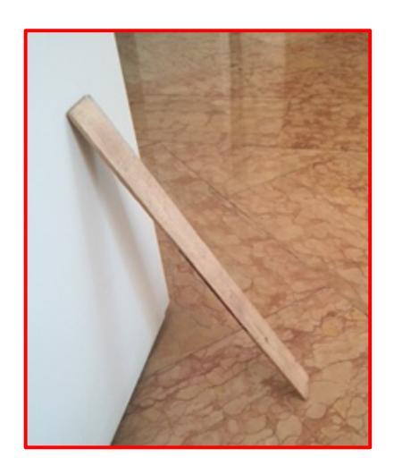
A ruler is leaning on a wall. How much can the ruler be inclined, before it just starts to move, if the coefficient of static friction between the ruler and the wall and the ruler and the floor are both 0.35?
