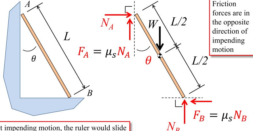
At impending motion, the ruler would slide down the wall and to right on the floor
