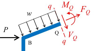
Three internal forces are developed to ensure equilibrium of each section
