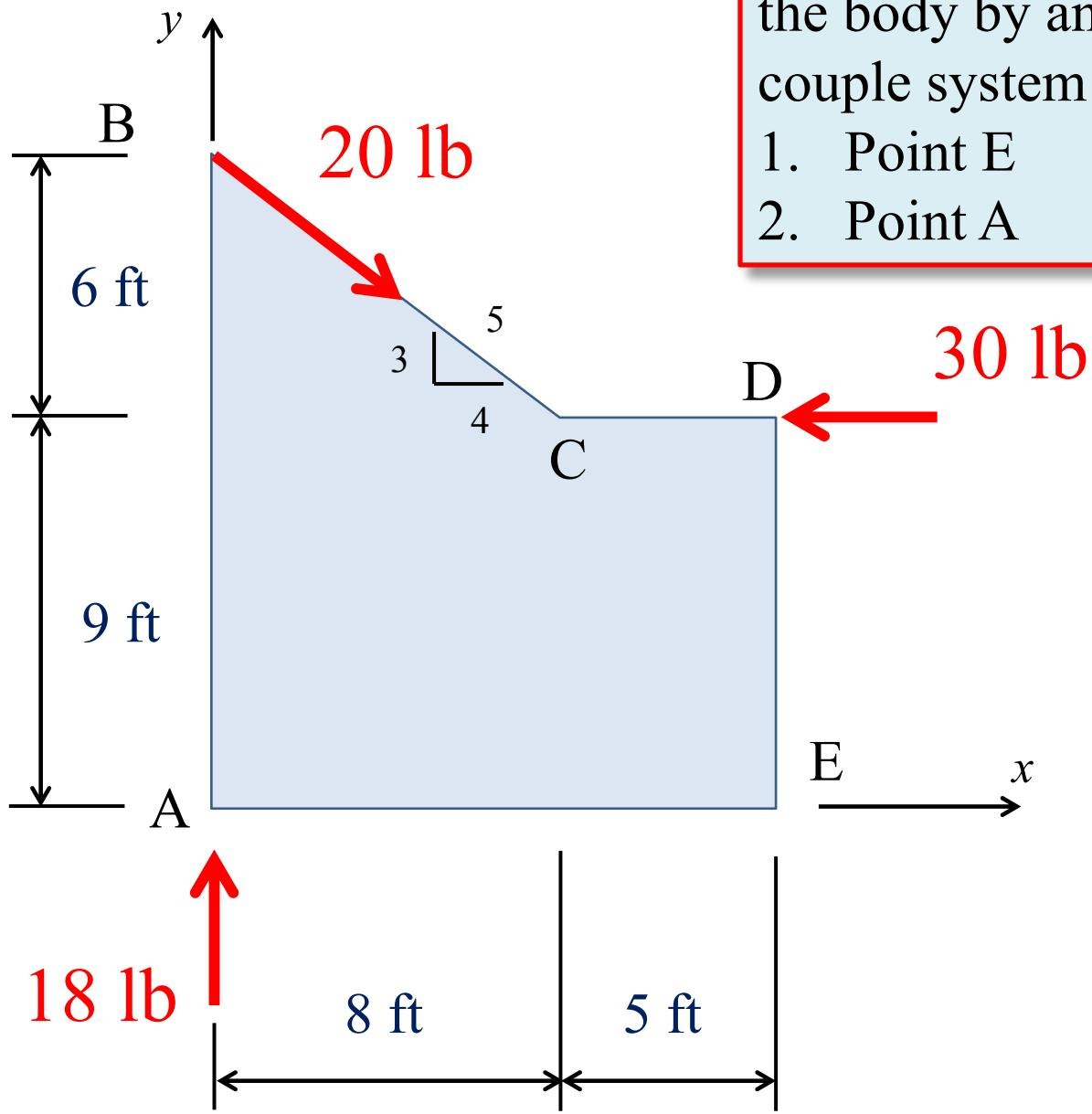
Replace the force system acting on the body by an equivalent force-couple system acting at:
