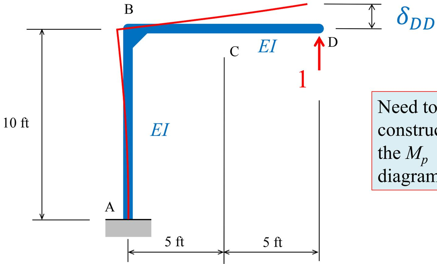
Need to construct the  $M_p$  diagram
