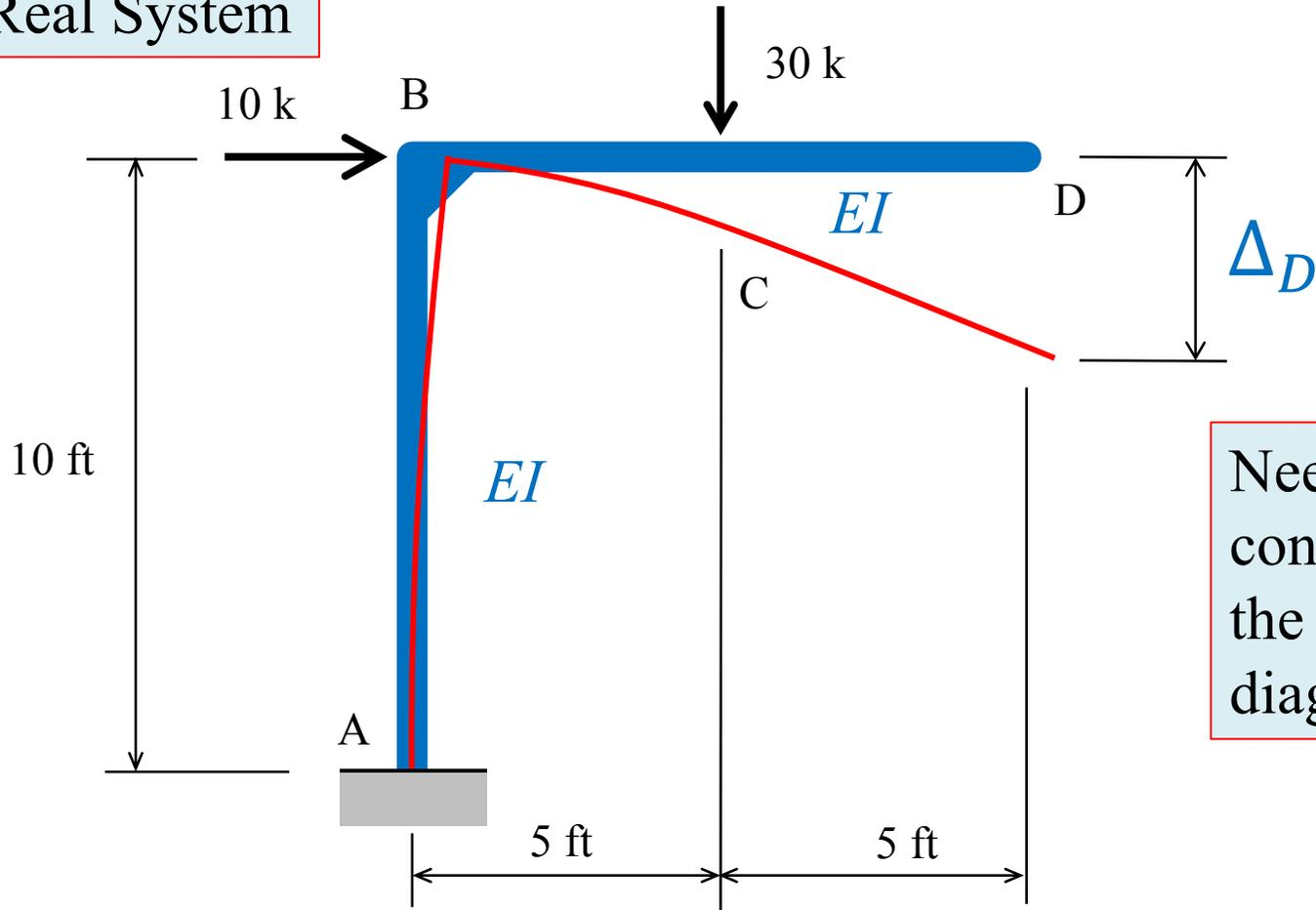
Need to construct the  $M_p$  diagram
