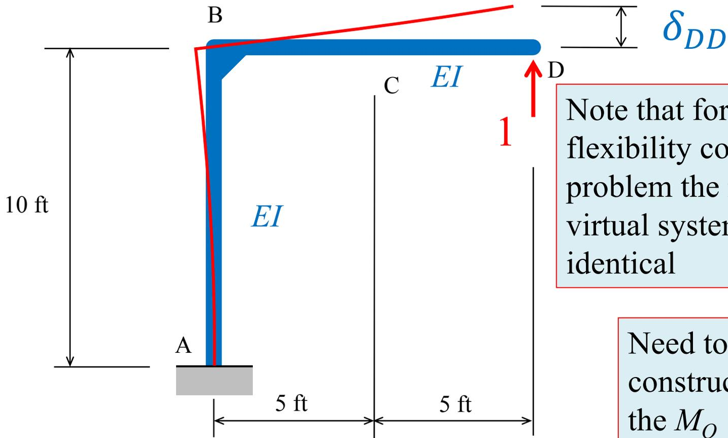
Note that for the flexibility coefficient problem the real and virtual systems are identical
