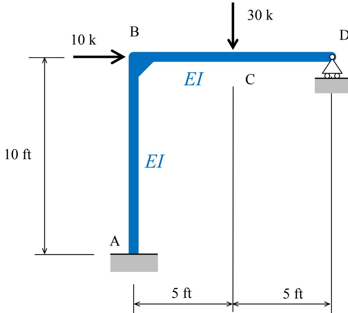
For the indeterminate frame subjected to the point loads shown, find the support reactions and draw the bending moment diagram for the frame.  $EI$  is the same for both the horizontal and vertical members.
