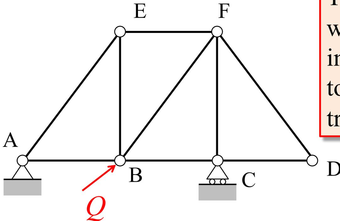
The virtual force will cause an internal axial force to develop in each truss member,  $F_{Qi}$
