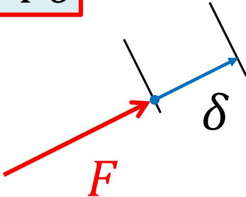
Work is done by a force acting through and in-line displacement
