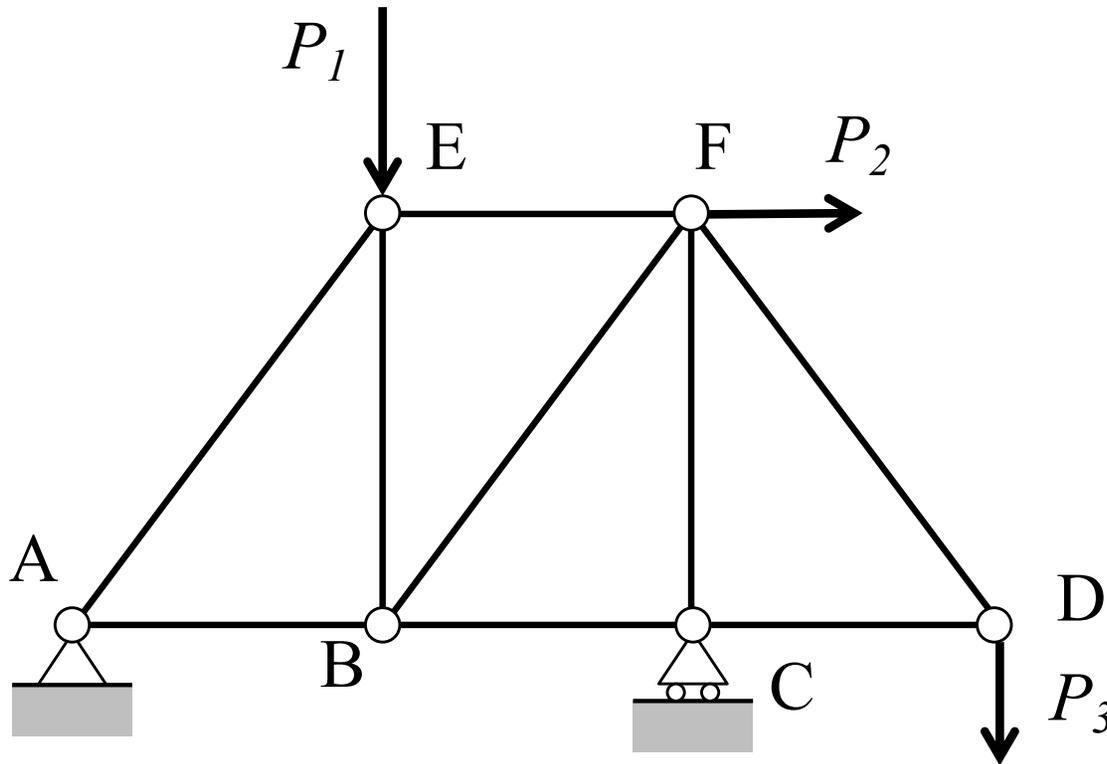
The real loads will cause an internal axial force to develop in each truss member,  $F_{Pi}$
