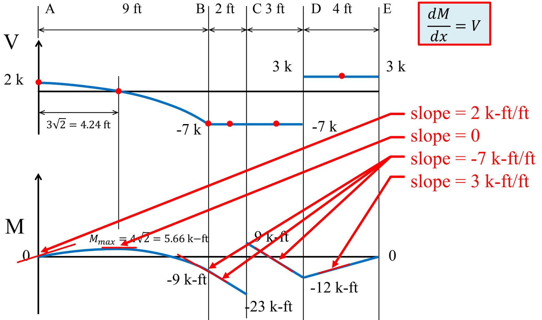
$$M_B - M_A = \int_A^B V dx = \text{area under the shear diagram between points A and B}$$
