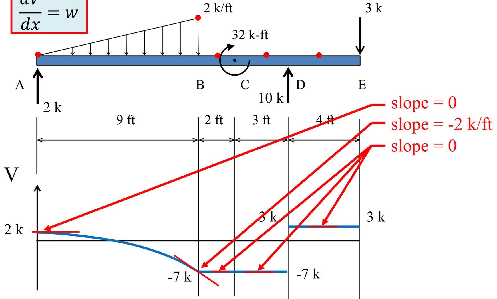
$$V_B - V_A = \int_A^B w dx = \text{area under the distributed load between points A and B}$$
