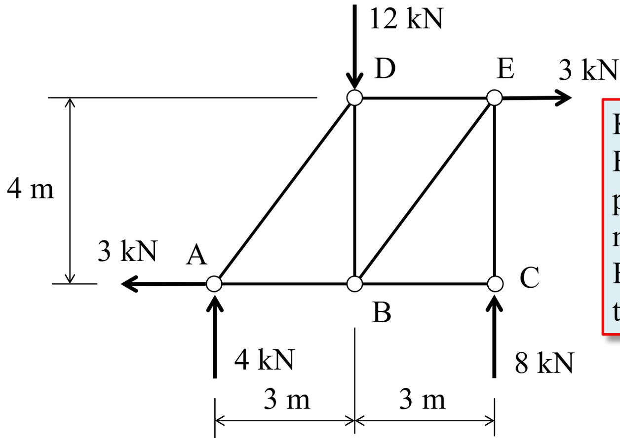
Knowing  $F_{CE}$  and  $F_{BC}$  from the previous analysis, now joints A and E are joints with two unknowns
