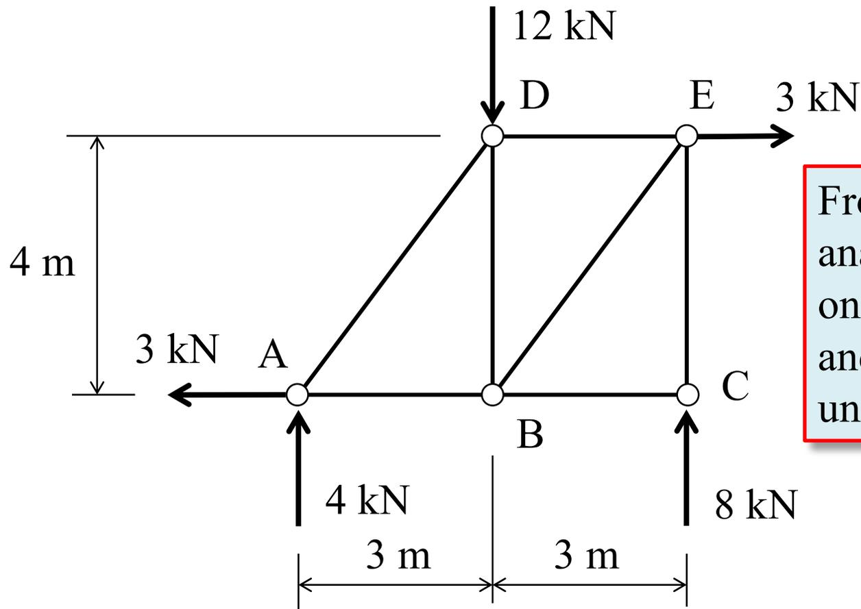
From the previous analysis, joint A has one unknown ( $F_{AB}$ ) and joint B has one unknown ( $F_{AB}$ ).
