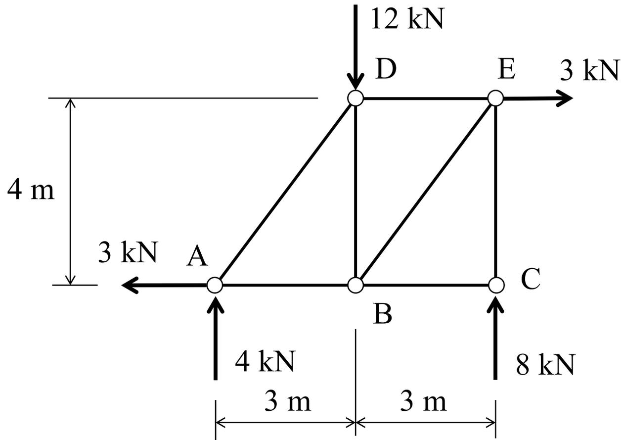
Knowing  $F_{CE}$ ,  $F_{BC}$ ,  $F_{DE}$ , and  $F_{BE}$ , from the previous analyses, now joints A, B, and D are joints with two unknowns
