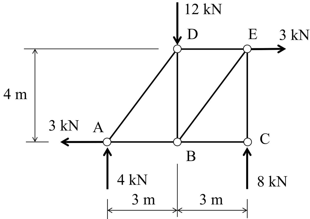
Joints A and C are the only joints with two unknowns
