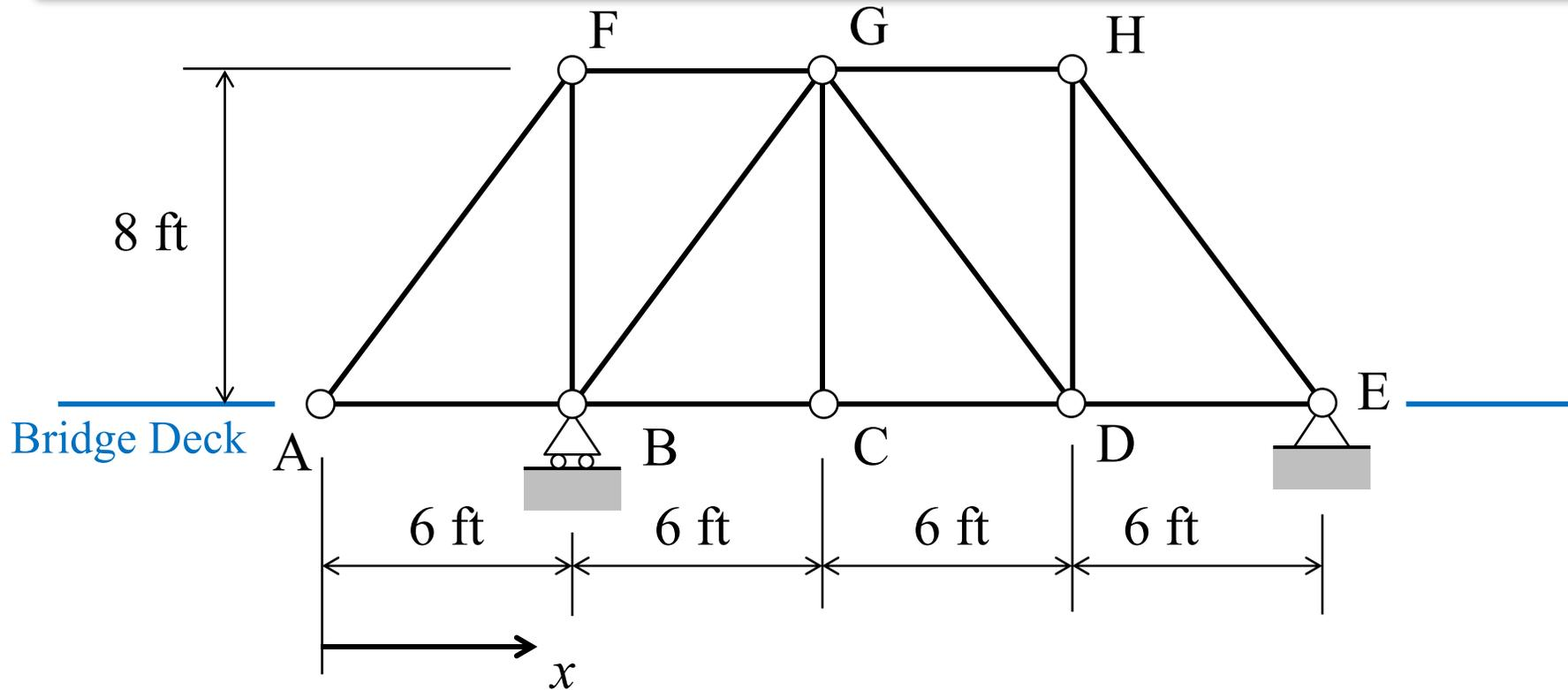
Unit load moves along level of bridge deck
