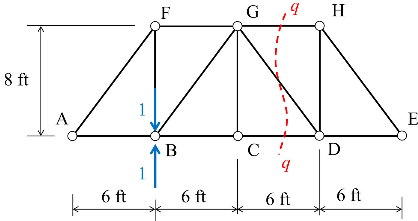
Note that for the unit load at roller support B, no axial forces are developed in any of the the truss members.
