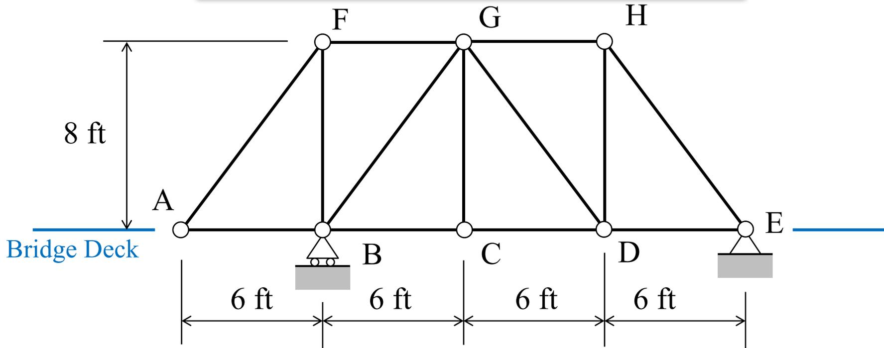
The truss shown supports a bridge deck and has a pin support at E and a roller support at B. For a load moving across the bridge deck, construct influence lines for:
