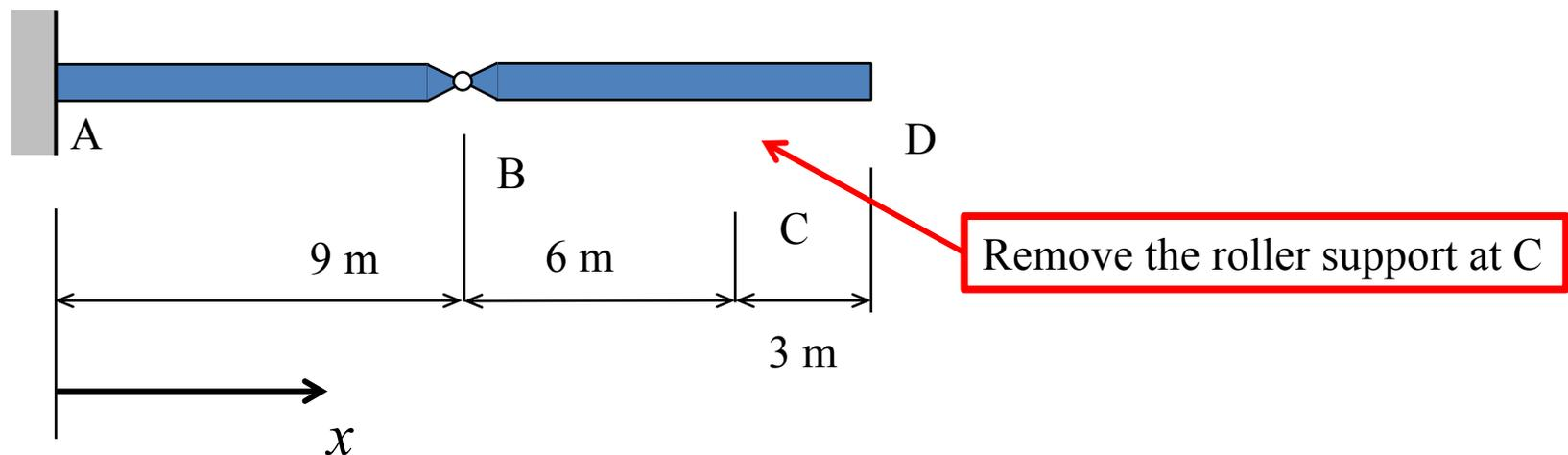
1. Remove the ability for the structure to resist the response quantity (e.g. reaction, internal shear, internal bending moment at a particular point). For a determinate structure this will result in an unstable structure.
