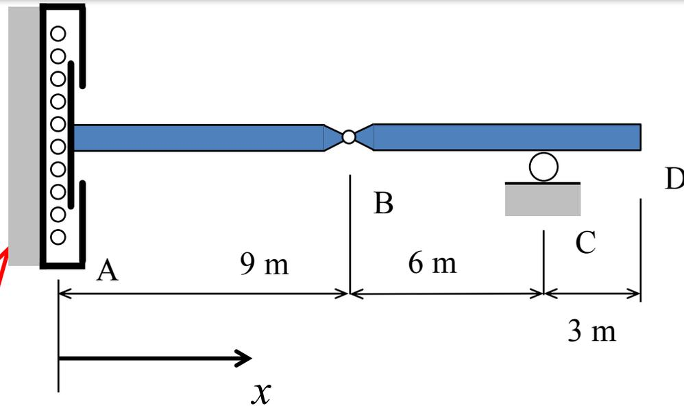
Remove the ability of the Support to resist vertical motion. Rotation is still restrained
