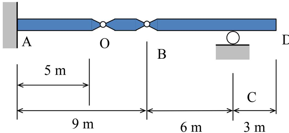
Remove the ability of point O to resist bending moment.
