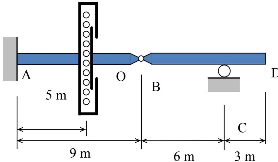
Remove the ability of point O to resist shear force.
