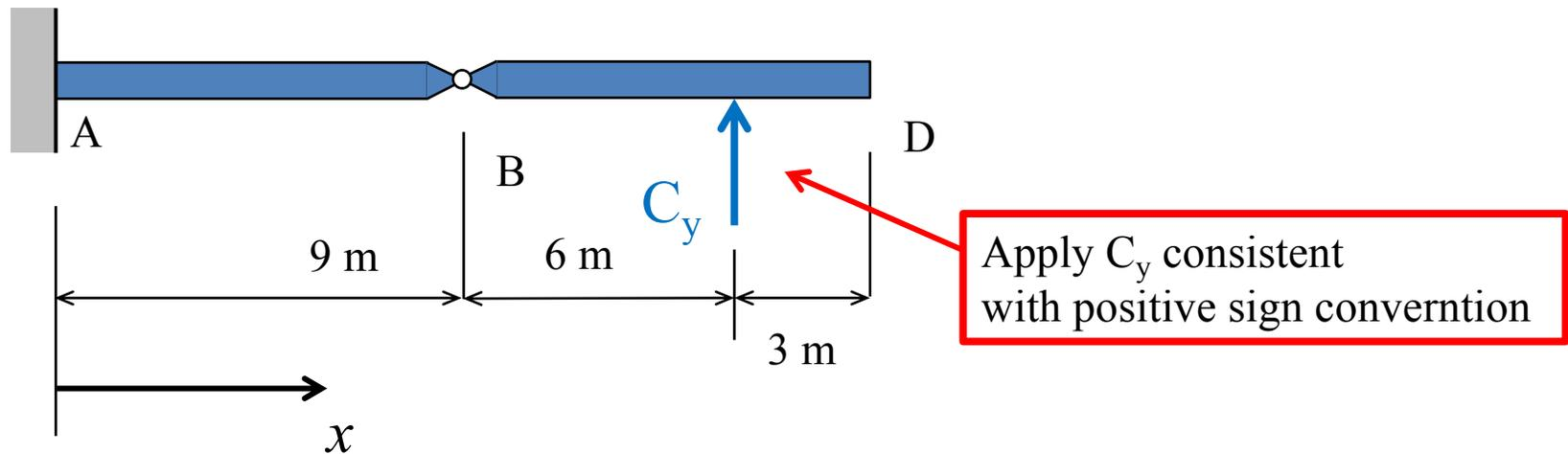
2. Apply the response quantity to the modified unstable structure from Step 1.
