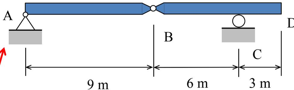
Remove the ability of the Support to resist rotation. Vertical movement is restrained
