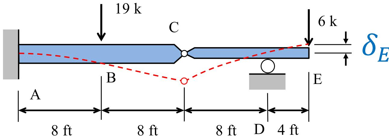
The overhanging beam shown has a fixed support at A, a roller support at C and an internal hinge at B.  $EI_{ABC} = 2,000,000 \text{ k-in}^2$  and  $EI_{CDE} = 800,000 \text{ k-in}^2$
