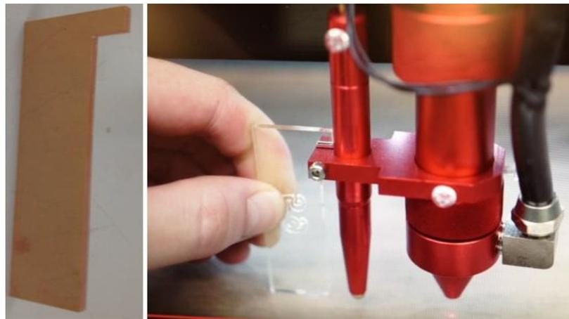
the **up** or **down** arrow button of the lower control touch screen panel shown in this picture. (Note that the arrows can only function when the file name has been selected, loaded and highlighted.) Be careful not to crash the laser nozzle on the workpiece. There is a lag, so you will have to hold the button down for a few seconds before it responds. Likewise, you will need to release it a few seconds before you want the head to stop moving.
