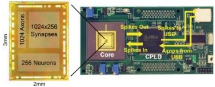
FIGURE 4: Neurosynaptic core and Board [1]
