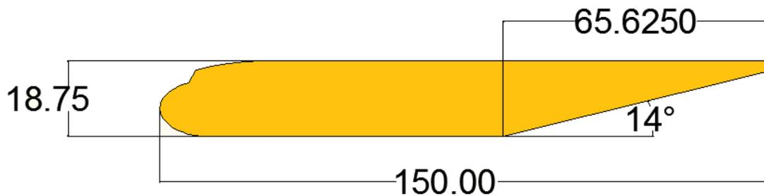
Figure6. 1 – General arrangement of the fuselage
