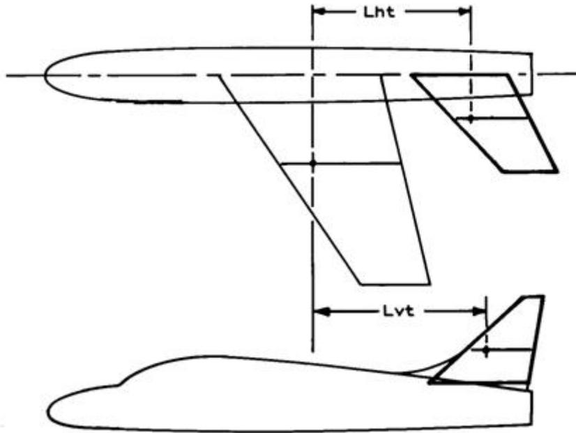
Figure8. 1 – Moment arm for the tail volume coefficient
