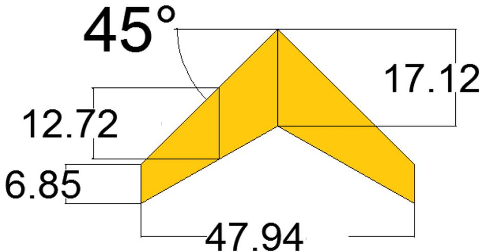
Figure8. 2 – CAD model for the horizontal stabilizer
