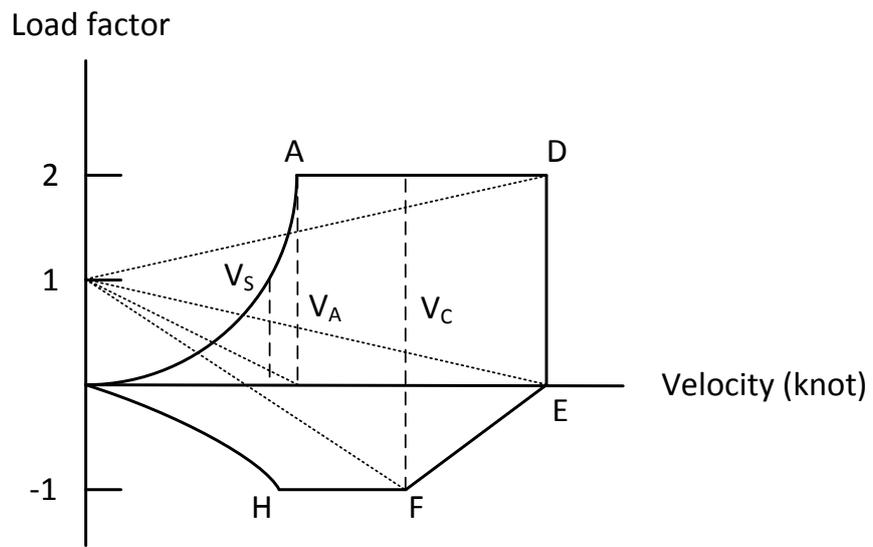
Figure13. 1 – V-N diagram for the KC-X
