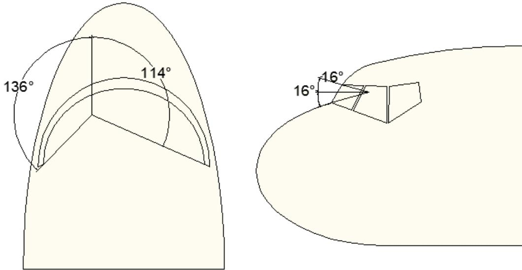
Figure6. 4 – Visibilities for the cockpit
