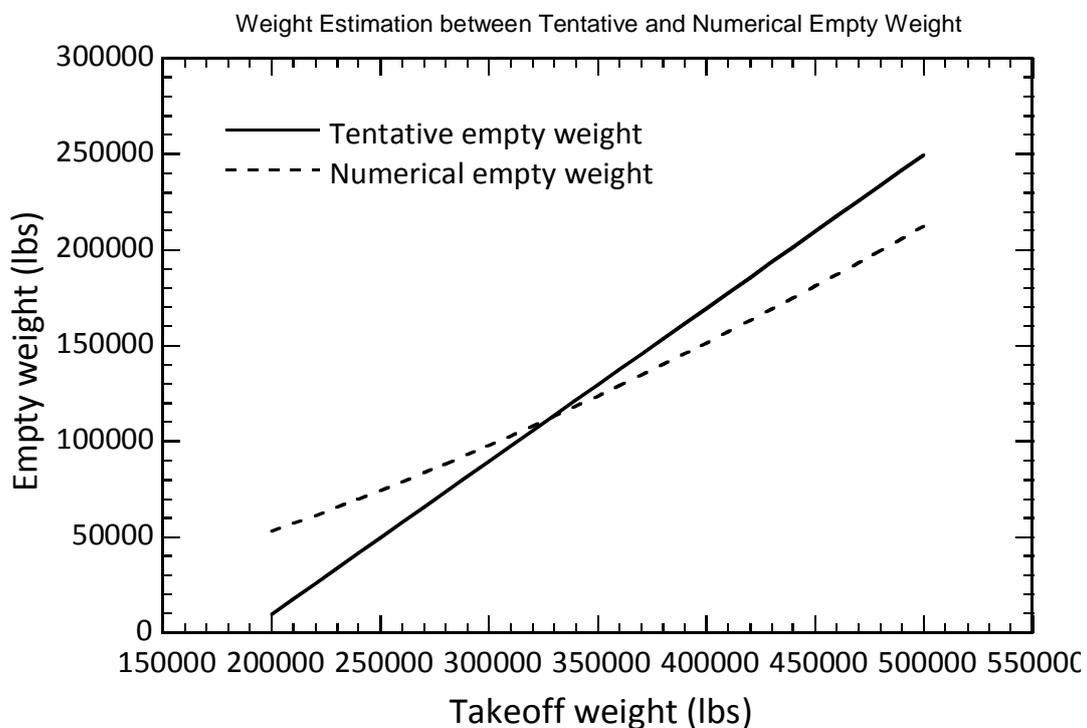
Figure4. 3 – Weight estimation between tentative and numerical empty weight
