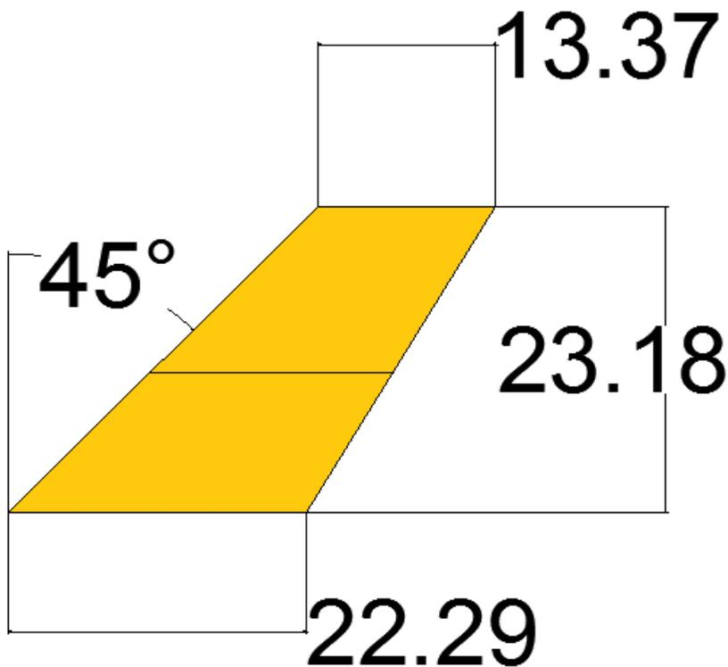
Figure8. 3 – CAD model for the vertical stabilizer
