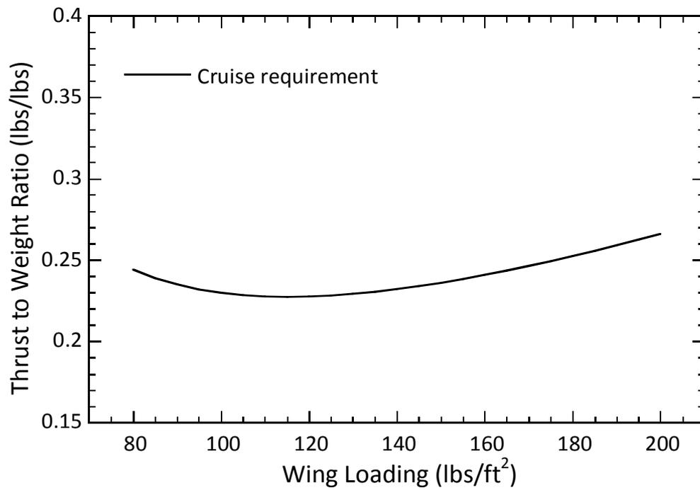
Figure5. 6 – Cruise speed requirement for aspect ratio 10
