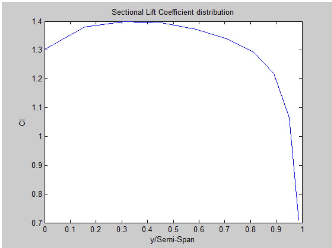
Figure 7.5 – 5 degrees angle of attack lift distribution
