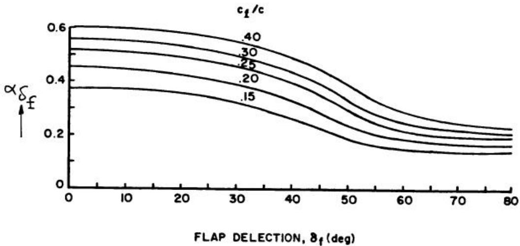
Figure 7.8 – Section lift effectiveness parameter for fowler flap
