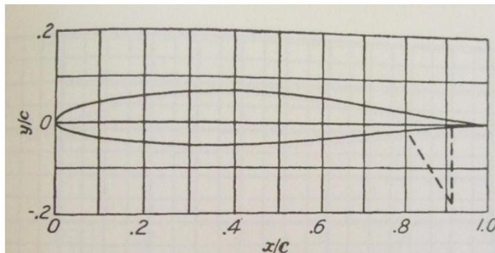
Figure7. 2 – NACA 641-212 airfoil
