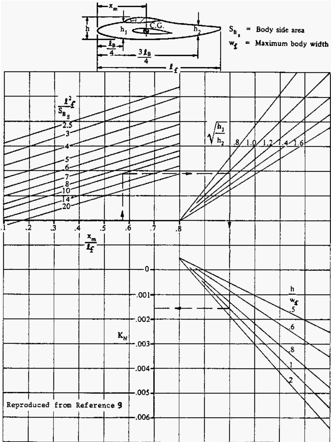
Figure 11.3 – Factor accounting for wing-fuselage interference with directional stability
