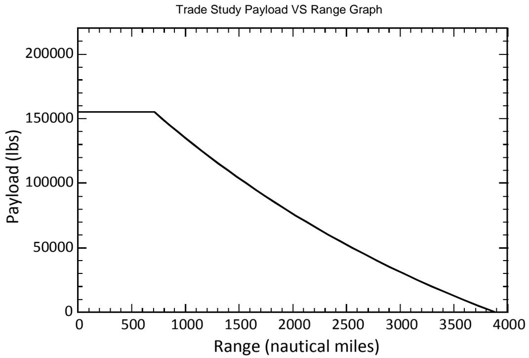
Figure4. 4 – Payload vs. range graph
