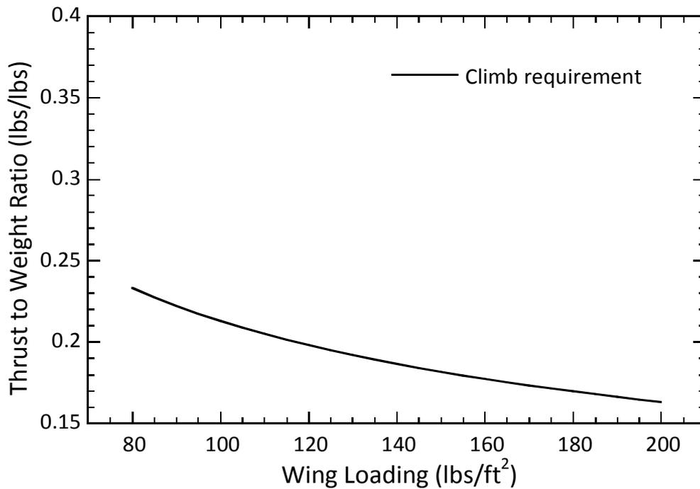
Figure 5.5 – One engine failure climb requirement
