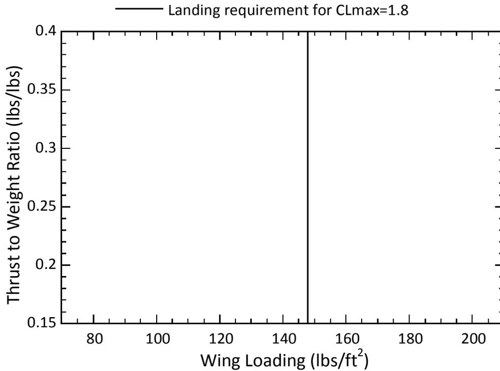
Figure5. 4 – Landing distance requirement for CLmax=1.8
