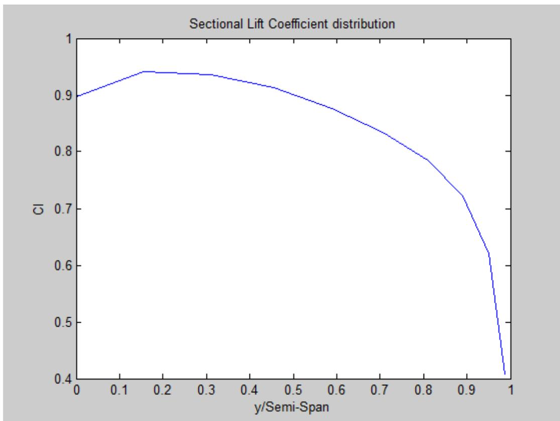
Figure 7.4 – Zero angle of attack lift distribution
