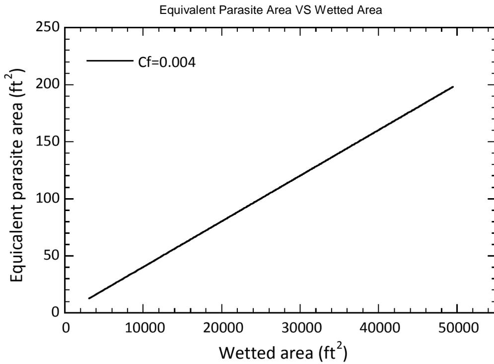
Figure5. 1 – Equivalent parasite area vs. wetted area
