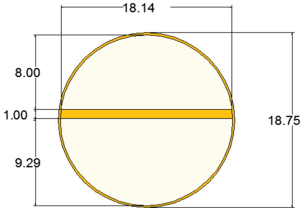
Figure6. 3 – Cabin cross section
