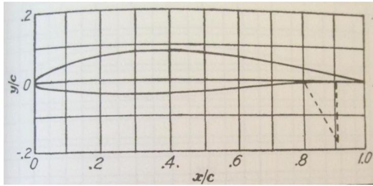
Figure 7.3 – NACA 641-412 airfoil
