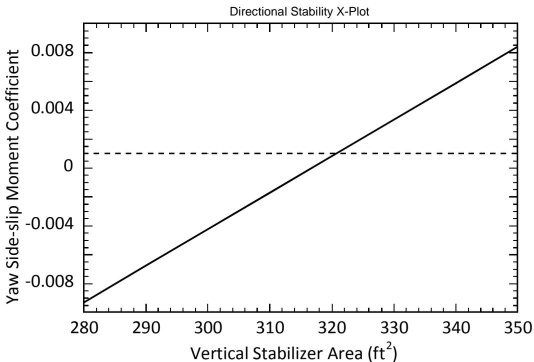
Figure11.2 – Directional stability X-Plot
