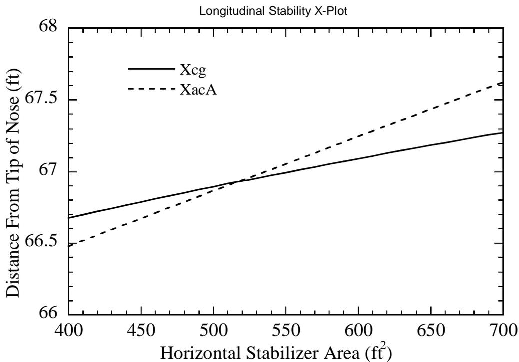
Figure11. 1 – Longitudinal stability X-Plot
