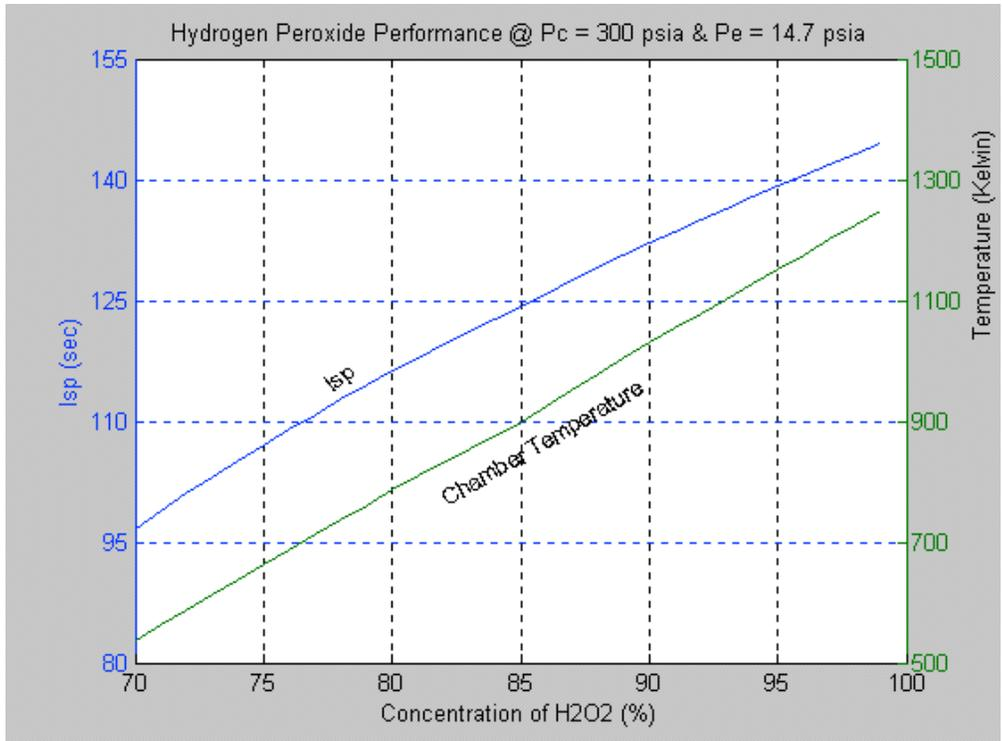
Figure 7 Concentration Effects on Hydrogen Peroxide Performance
