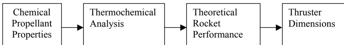
Figure 1 Chemical Rocket Preliminary Design Flow Chart
