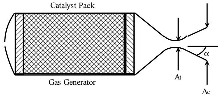
Figure 2 Nozzle Dimensions, Low Thrust Application
