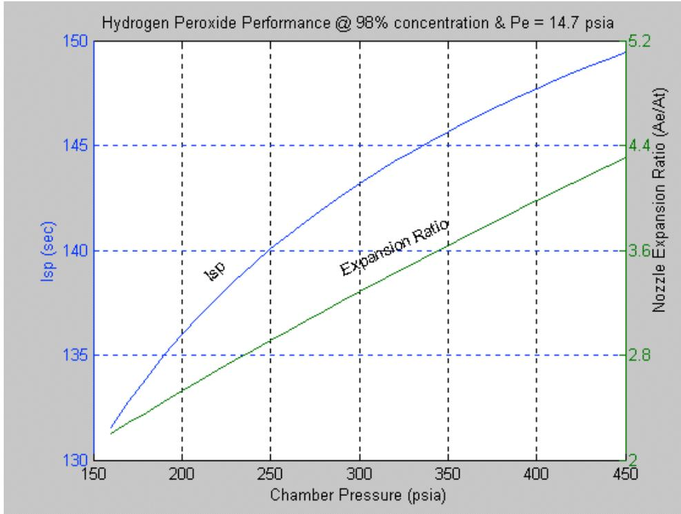
Figure 8 Chamber Pressure Effect on Hydrogen Peroxide Performance
