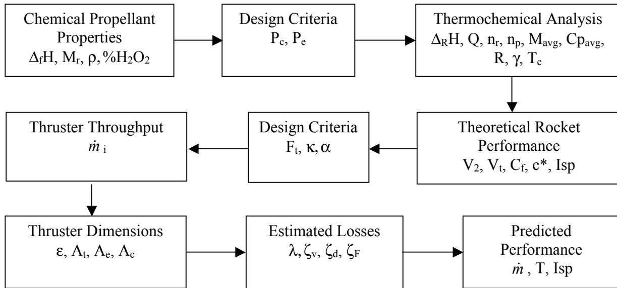
Figure 4 Computer Program Flow Diagram
