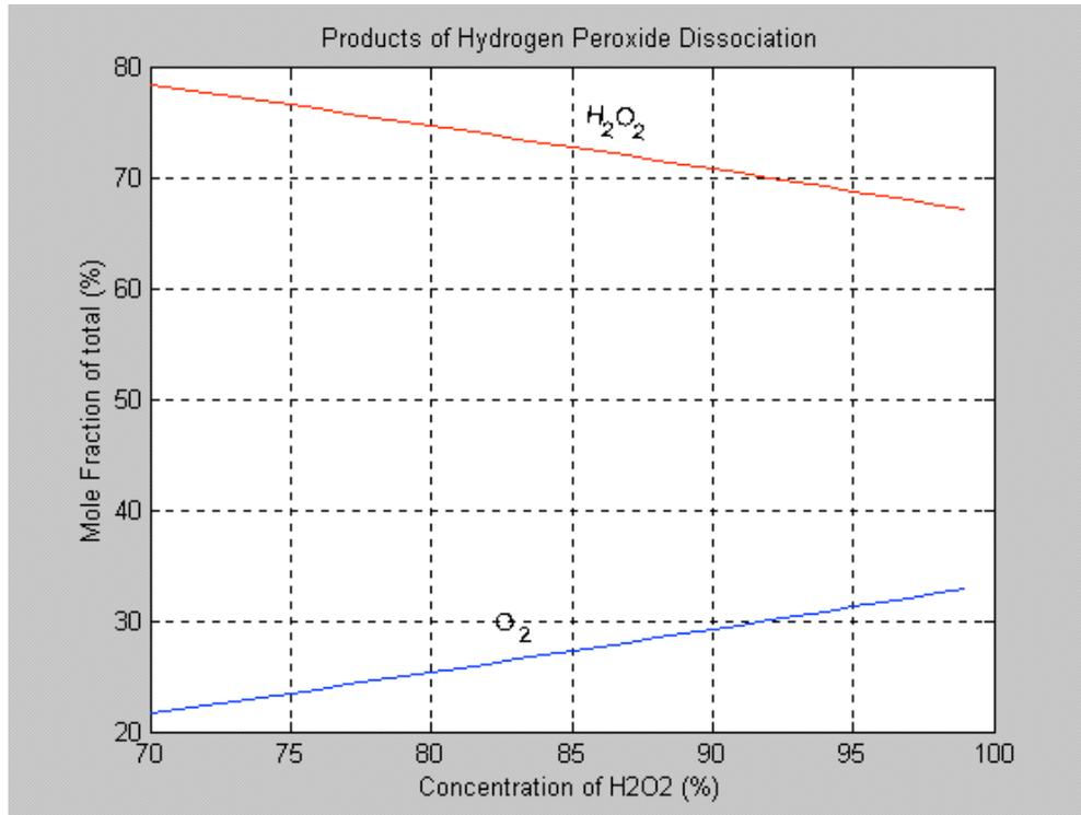
Figure 6 Hydrogen Peroxide Reaction Products
