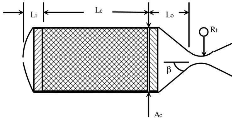
Figure 3 Empirically Determined Thruster Dimensions
