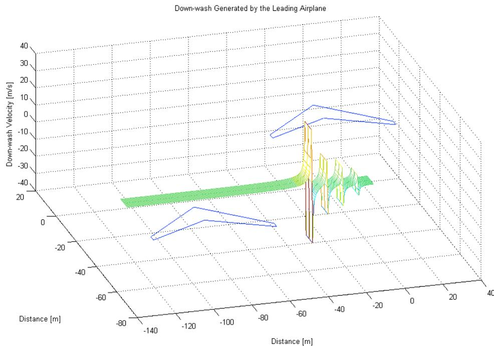
Figure 2.2 **Downwash** and **upwash** due to the leading airplane.
