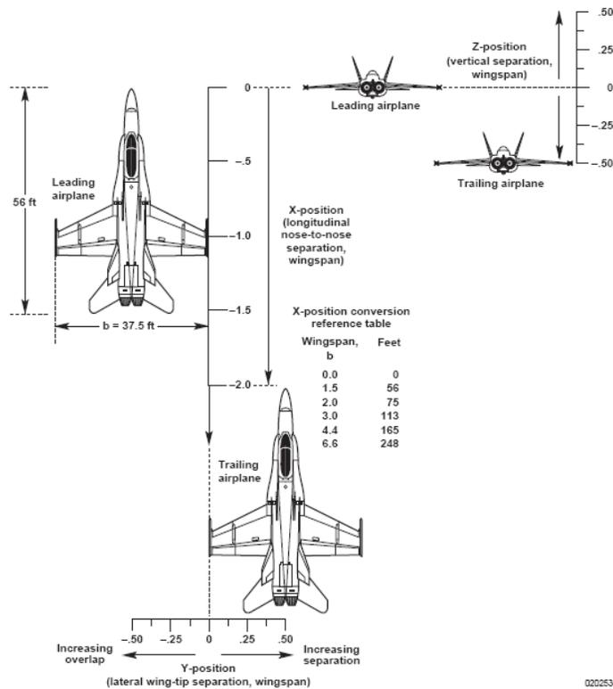
Figure 2.5 Relative coordination in formation **What kind of formation is this?** (Vachon, M. J. et al. 2003).
