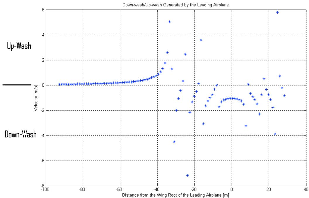
Figure 2.3 Down-wash and up-wash due to the leading airplane at one wing span behind
