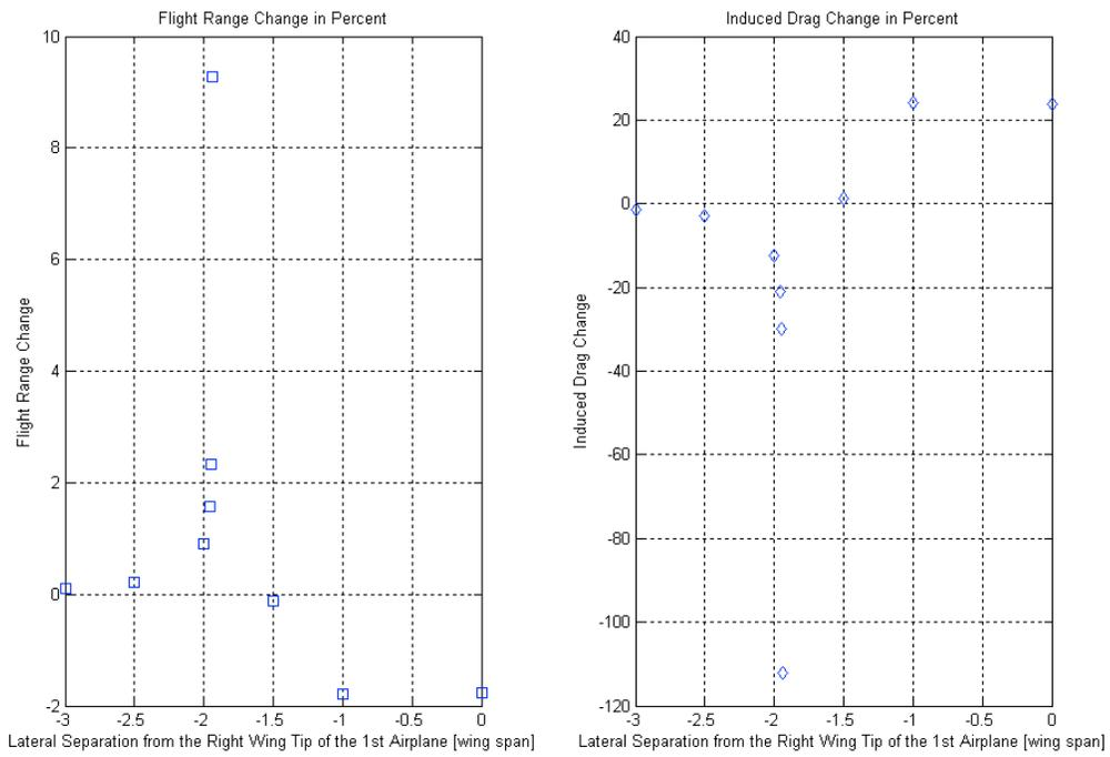
Figure 5.4 Change of induced drag and flight range at different positions of 4<sup>th</sup> airplane in the five-airplane formation.
