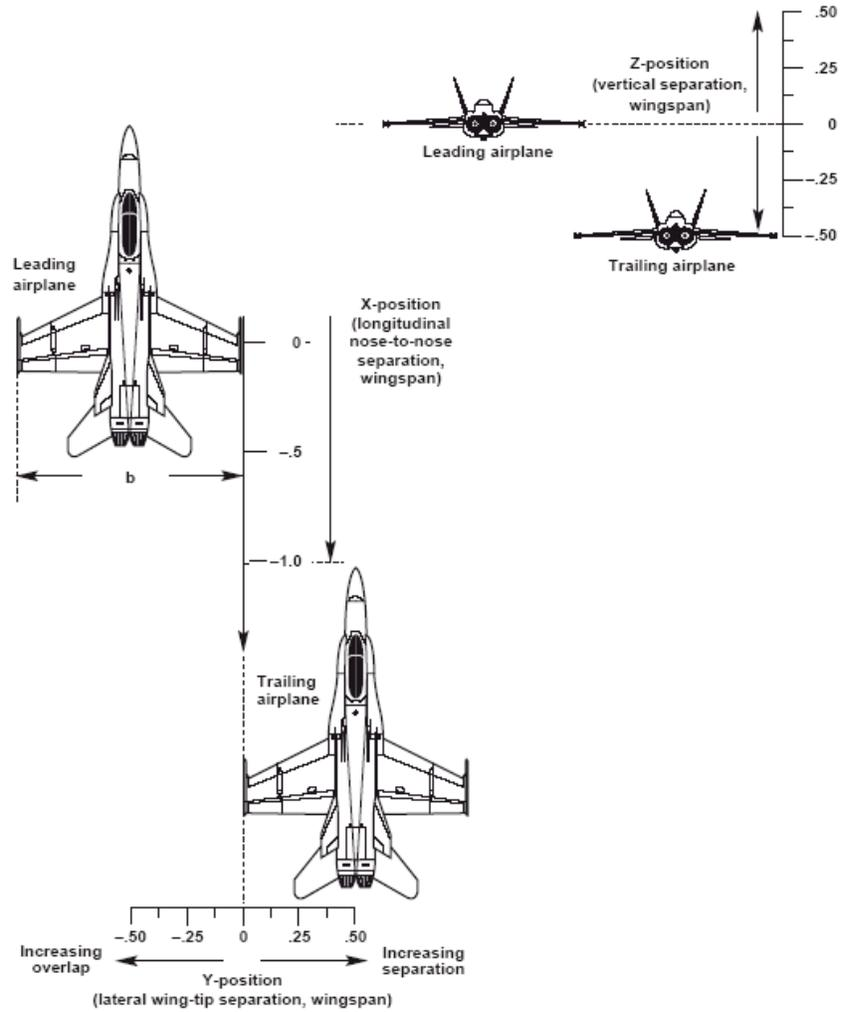
Figure 5.1 Relative coordination in formation (Vachon, M. J. et al. 2003).
