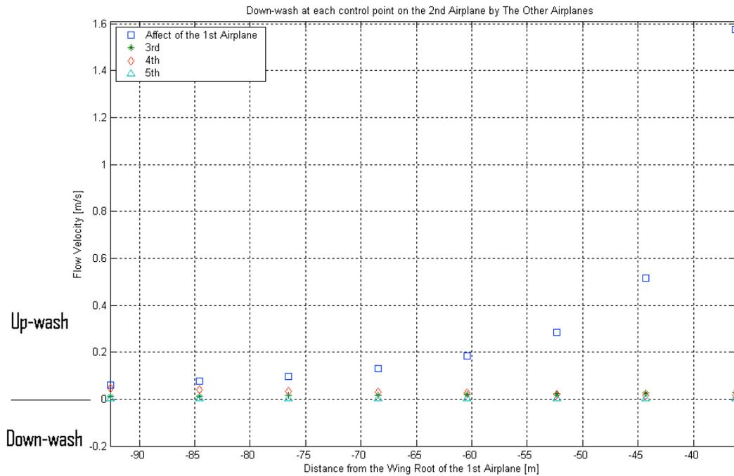
Figure 5.3 Down-wash contributions at each control point of the 2<sup>nd</sup> airplane.
