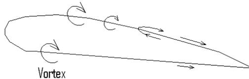
Figure 3.1. The Arrangement of Vortices over the Airfoils.
