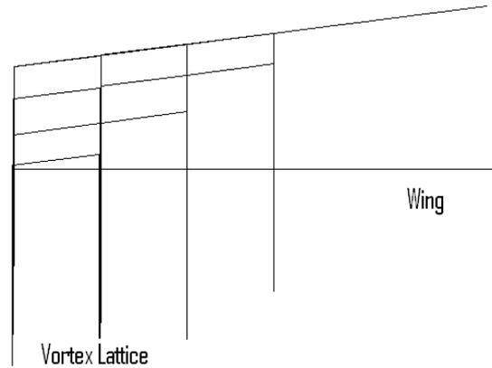
Figure 3.2. The Arrangement of Vortices over the Wings in the Vortex Lattice Method
