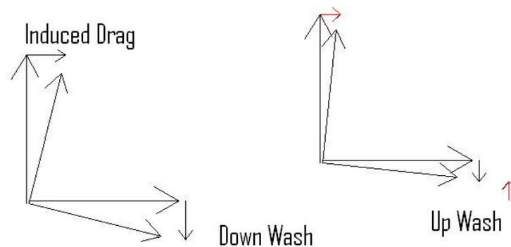
Figure 2.4 Induced drag, down-wash and up-wash.
