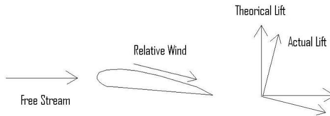
Figure 2.1. Relative Wind over the airfoils.
