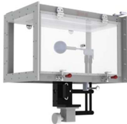
**Figure 3.2 - AEROLAB Wind Tunnel Test Section (AEROLAB, 2007)**
