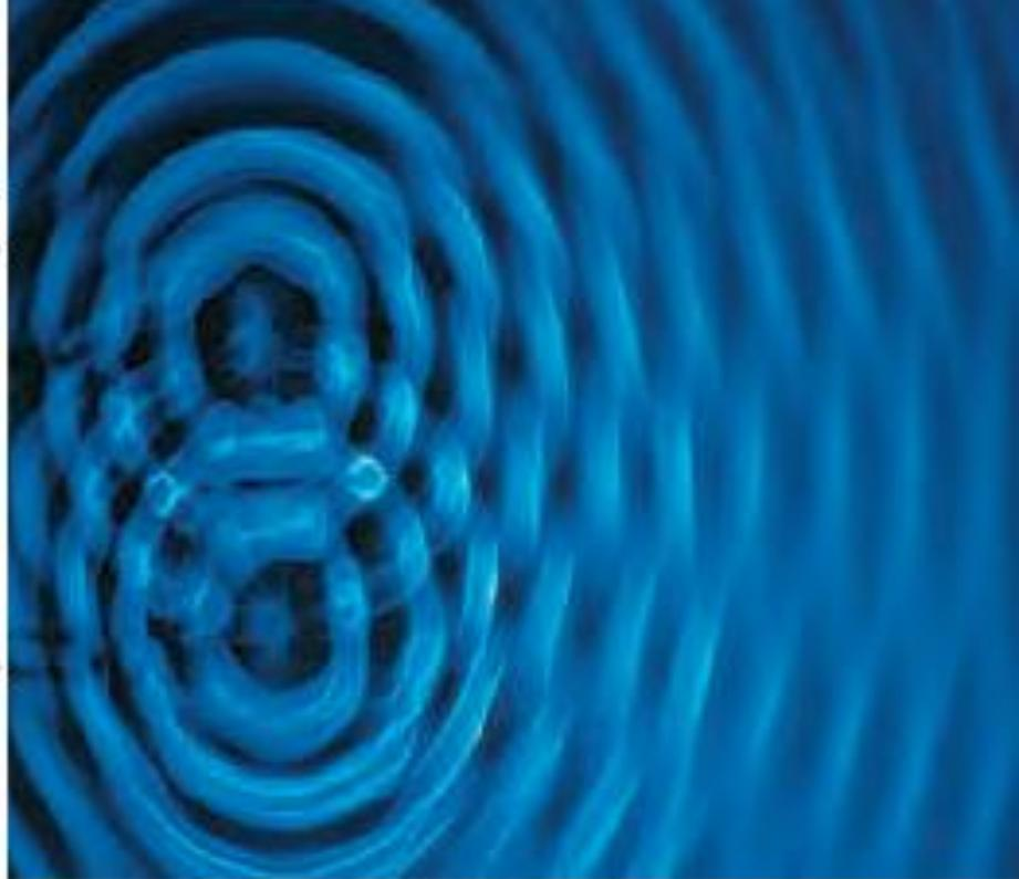
**Figure 24.2** An interference pattern involving water waves is produced by two vibrating sources at the water's surface. The pattern is analogous to that observed in Young's double-slit experiment. Note the regions of constructive and destructive interference.
