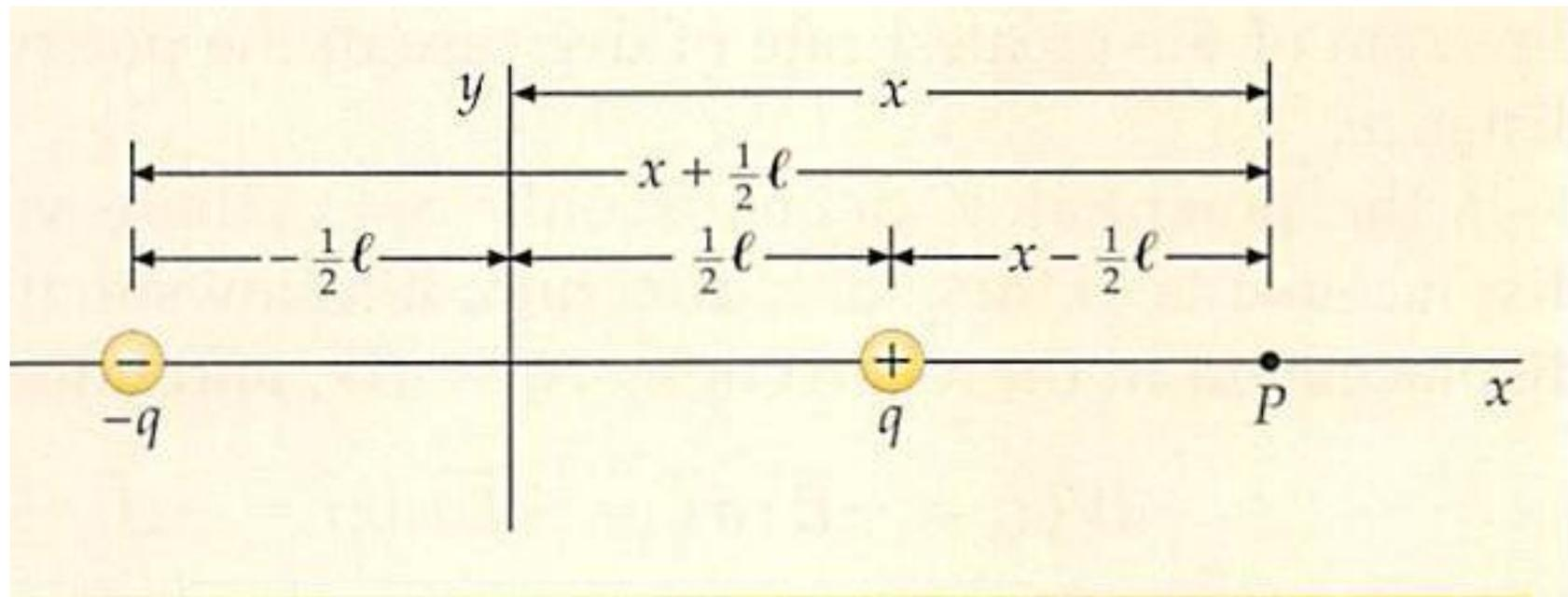
Sketch the  $x$  axis and place the two charges on it. For  $x > \ell/2$ , the distance from the field point  $P$  to the positive charge is  $x - \frac{1}{2}\ell$  and the distance from the field point to the negative charge is  $x + \frac{1}{2}\ell$
