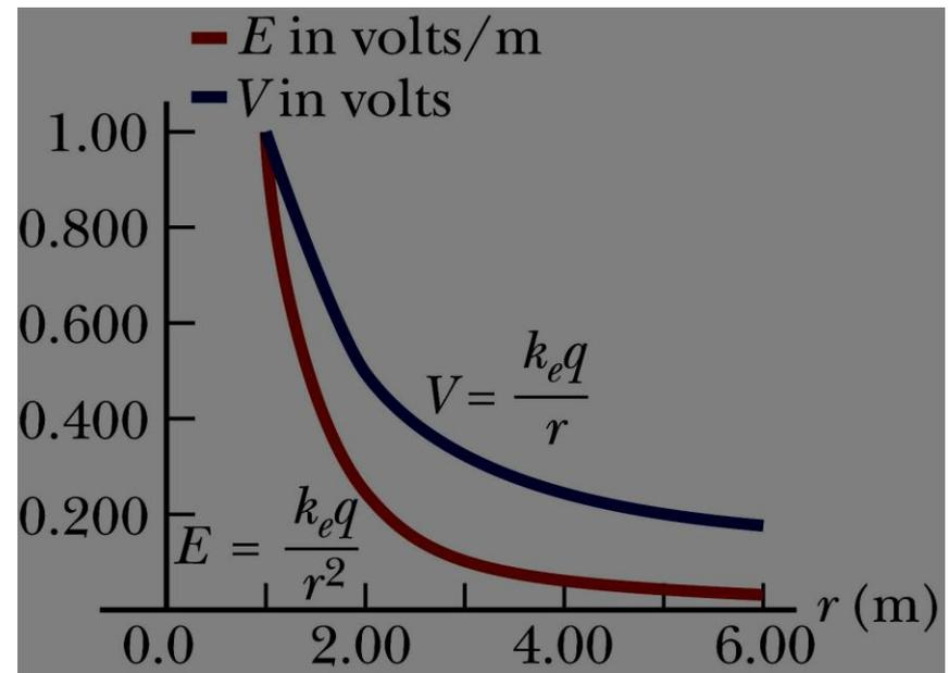
If the conservative force is exerted by electrostatic field  $E$  on point charge  $q$ , then the force is given by
