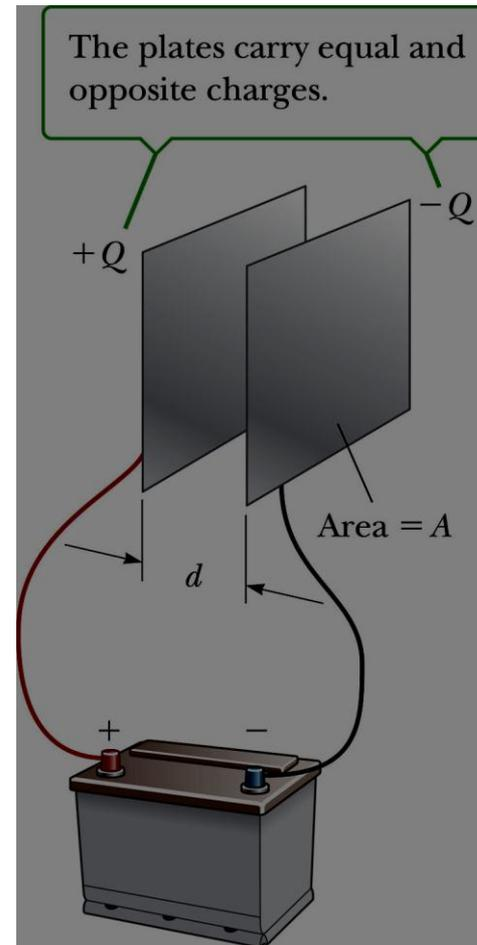
The capacitance  $C$  of a capacitor is the ratio of the magnitude of the charge on either conductor (plate) to the magnitude of the potential difference between the conductors (plates):
