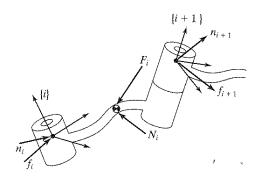
Force and torque balance equations at the center of mass of link i:
