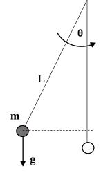
$$\frac{\delta L}{\delta \theta} = -mgl\sin\theta \qquad \frac{\delta L}{\delta \omega} = ml^2 \omega \qquad \frac{d}{dt} \frac{\delta L}{\delta \omega} = ml^2 \dot{\omega}$$
